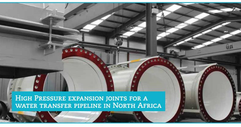
MACOGA has completed the production of 6 units High Pressure Universal Untied Reinforced expansion joints MFD Series DN1800 and DN1000.
