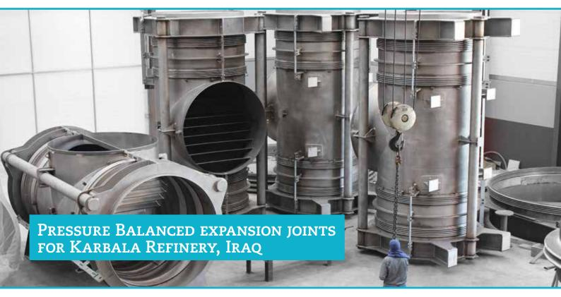
MACOGA has successfully designed, manufactured and tested 4 units large Pressure Balanced expansion joints DN2200 and 8 Lateral tied units DN1600 for Karbala Refinery Project in Iraq.
