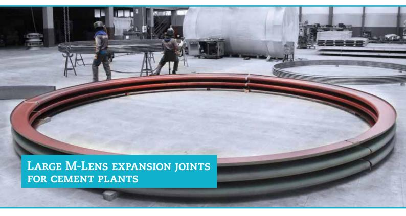
MACOGA has successfully designed, manufactured and tested very large M-Lens expansion joints NB 5400, NB 2600 and NB 1200 for cement plants.
